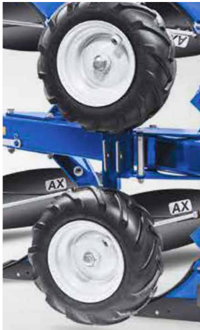
Dual wheel - 23x8.50-12 BX, CX, side mounted
