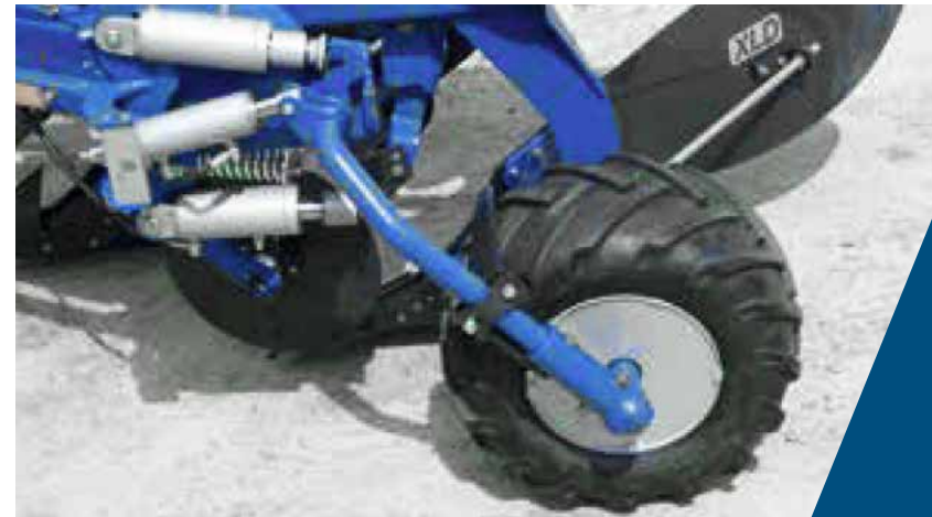
Hydraulic depth control and rim sides for tractor pattern support wheel.
